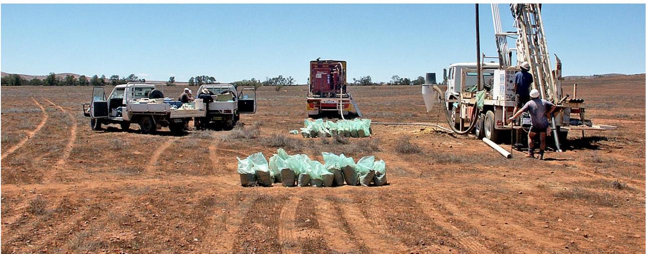
Figure 1 Drill rig at site 80a (Mookkra area) where a 2.5 metre wide kimberlite dyke was located in two holes.
