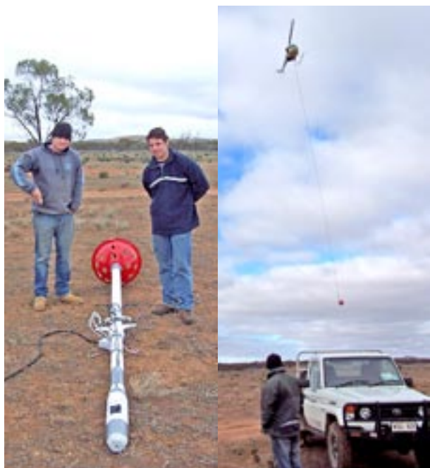
Figure 4 Helimag survey July 2005, from left, Ryan Greenhalgh and Andrew Aouad with magnetometer bird, helicopter taking off with bird to commence survey.
