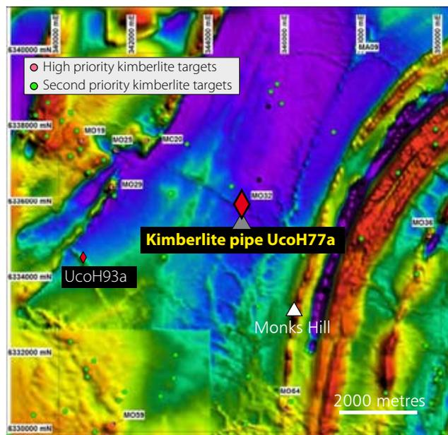
Figure 2 Pipe and fissure targets in the Monks Hill area with the Helimag image in the background.
