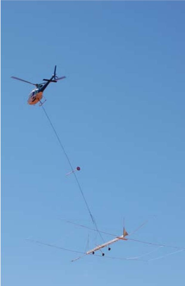
**Figure 2** Electromagnetic loop slung below helicopter during surveying.
