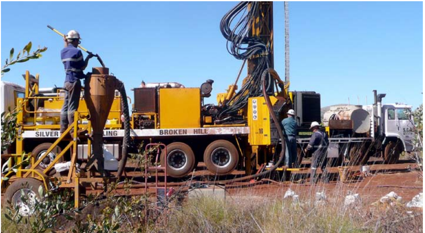
Figure 3 Silver City Drilling carrying out RC drilling on hole HRC12.
