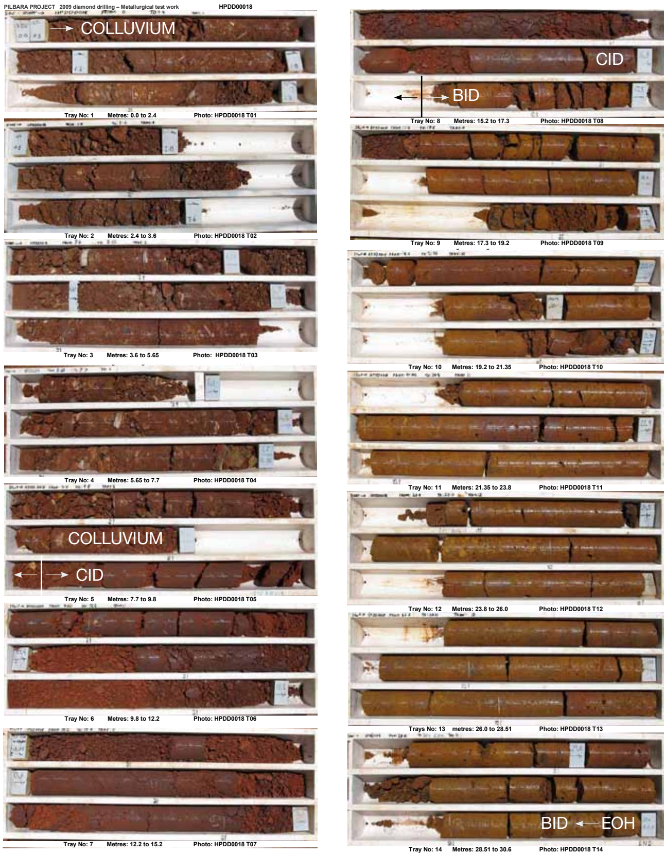
Figure 4 Core trays from diamond drillhole HPDD0018 in Delta Prospect showing examples of CID and BID mineralisation to be used for metallurgical testing (see Figure 4).
