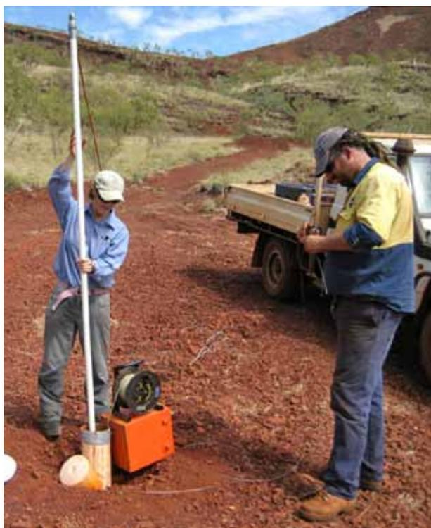
*Measuring borehole water levels during hydrological surveying, Pilbara Iron Ore Project, November 2009.*
