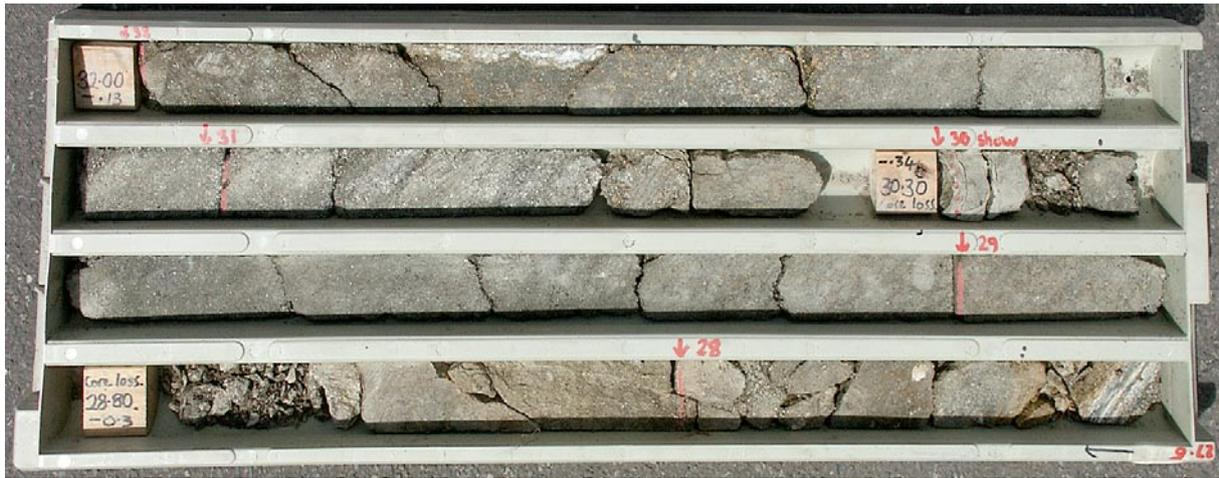
**Photo 4** Vermiculite rich Bleechmore drill core from 27.5 to 32.0 metres in hole BD1.
