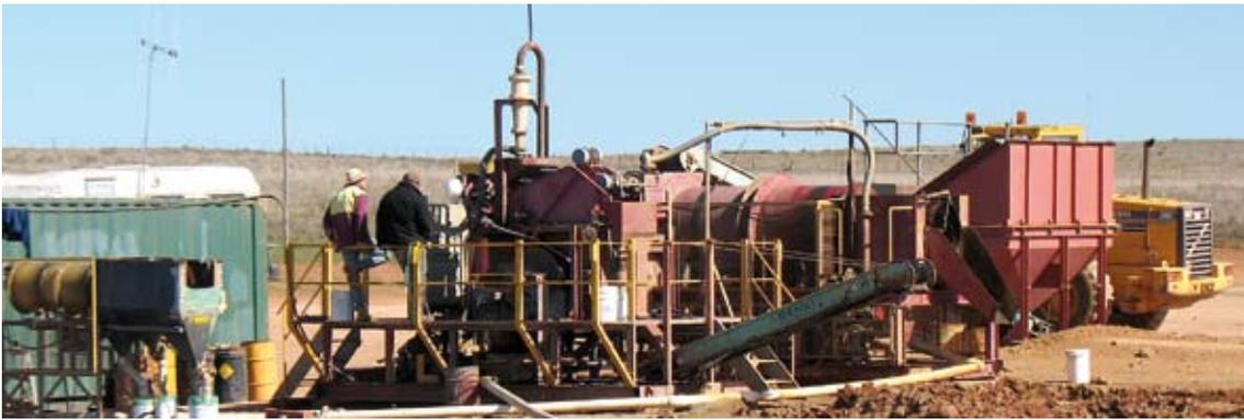
Figure 2 Dense media separation section of the bulk sampling plant near Terowie, South Australia.
