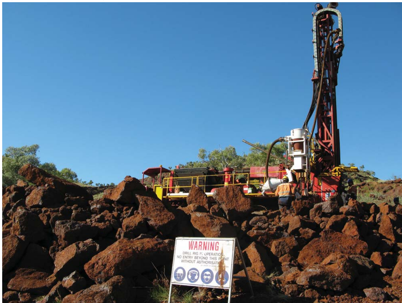
Figure 2: Reverse circulation drilling on the north-eastern flanks of Delta deposit, 2013.
